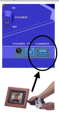
Figure 14 – Connecting a Camera
